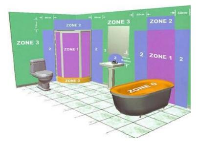
Jeeves heated towel rails are therefore certified for installation in Zone 1 which includes the area above the bath.
