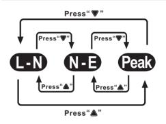
Voltage (Vd): real time display of cable connection status and display the voltage drop of current load and measurement results of phase voltage drop TRMS. This test item includes 3 submenus, namely load with 5A, 8A and 10A. Press Up " (a)" or Down " (b)" selection key on the sub test item to enter the relevant test item.
